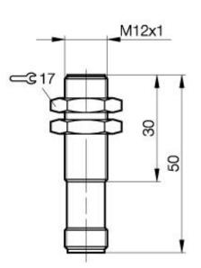
Inductive Sensors BES 515-325-E5-T-S 4 M12x1 x 50 normally-open Sn=2mm shielded
